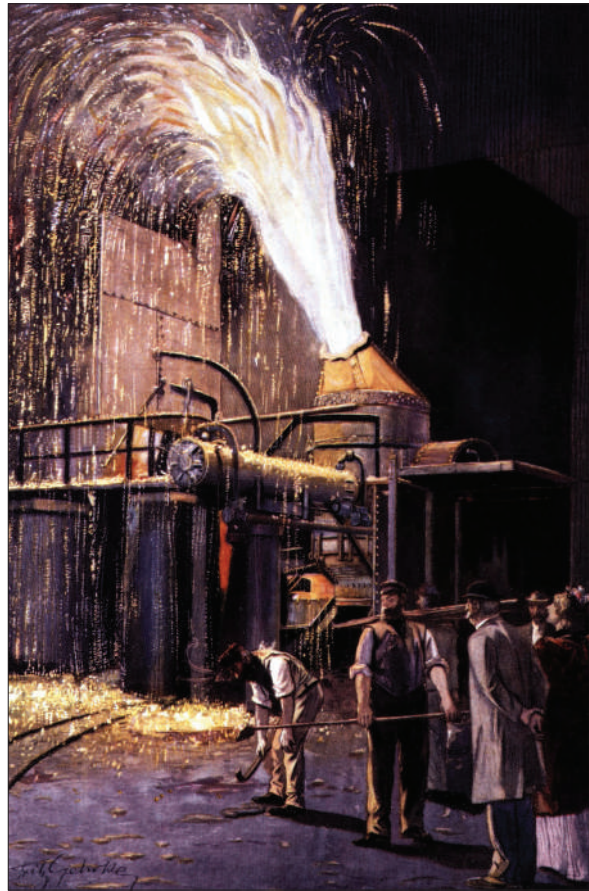
The Bessemer process revolutionized the global steel industry. Between 1880 and 1890, steel production in the United States increased an astonishing 290 percent.
