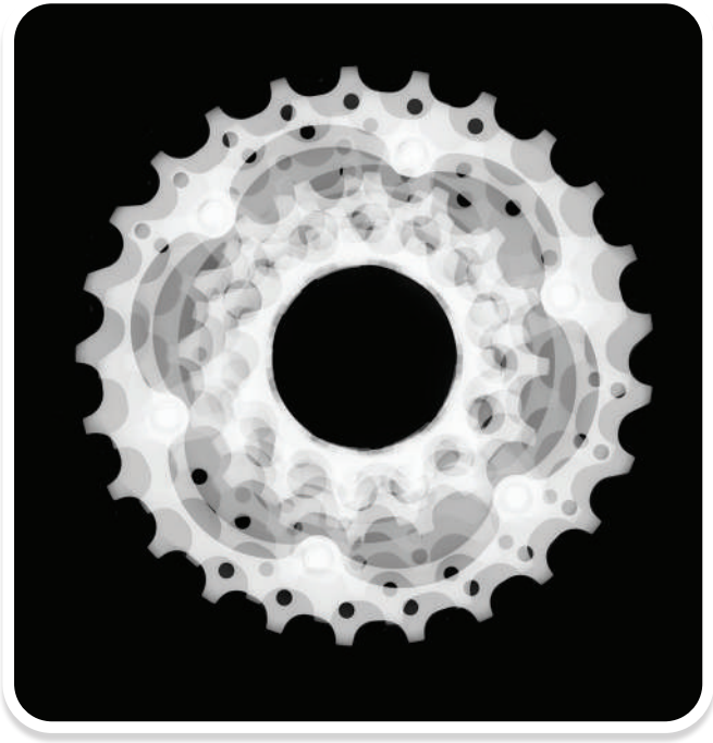
This image shows x-rays of a bicycle gear. Scientists used x-rays of the Antikythera mechanism's gears to learn more about how it worked.
