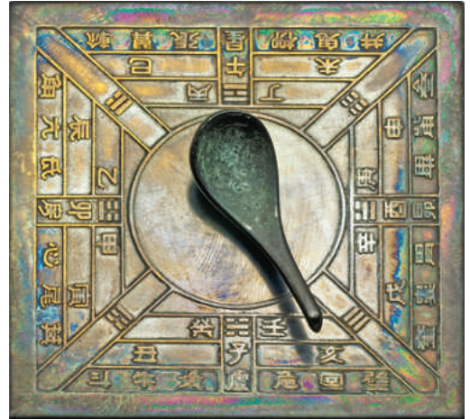
In early versions of the compass, the magnetic stone was shaped like a spoon and moved on the bronze dish below it.
