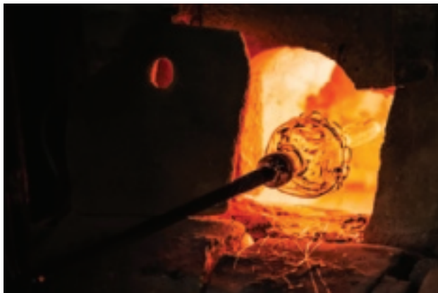
Sand being melted at a high temperature to make glass
